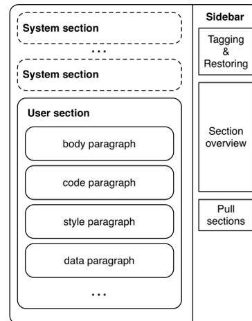
**Figure 2.** A schematic overview of the structure of a codestrate. On the left are sections, which include system sections (hidden by default) and one or more user sections. Sections can include paragraphs of different types (body, code, style, data). On the right is a sidebar (hidden by default), which contains actions for the codestrate (create a copy of the codestrate, tag and restore, pull from another codestrate) and actions for the sections (toggle sections' visibility, add section).
