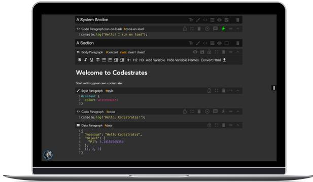
Figure 5. Codestrate view of Listing 1, including paragraphs and their contents. The section containing the bootstrap code is hidden.
